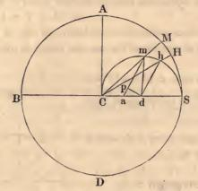
Let A B D S be a great circle, S and M the places to which the sun and moon are vertical; on S C, as diameter, describe a circle, bisect S C in (d); and take S d : d a :: M : S. Take the angle S C M =  $(\varphi + \theta)$ , and let C M cut the inner circle in (m), join (m a) and draw (h d) parallel to it; through (h) draw C h H meeting the outer circle in H; then will H be the place of high water.
